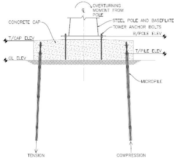
Figure 1: Micropile Tension and Compression
