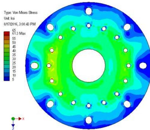
Figure 6: Autodesk Inventor Output Showing Localized Stresses at the Surface of a Cap
