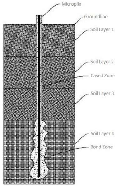
Figure 2: Micropile Installation Schematic
