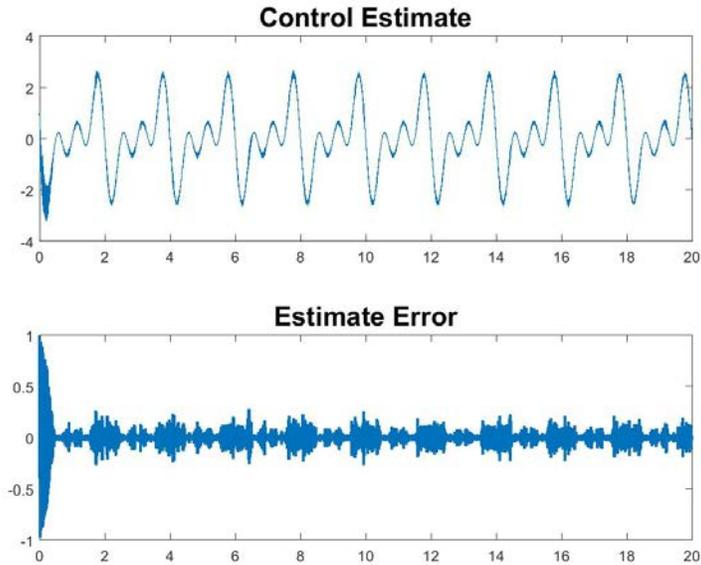
Figure 6: Reconstructed Signal and Estimate Error with Robust Control
