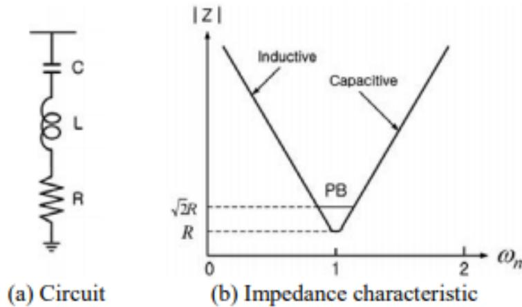
Figure 7: Passive Tuned Harmonic Filter Circuit and Impedance Characteristics
