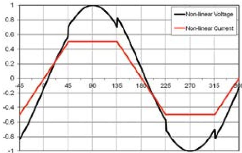
Figure 2: Non-linear Voltage and Current
