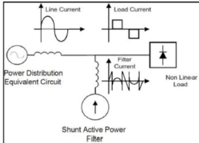
Figure 8: Active Harmonic Filter and Waveform
