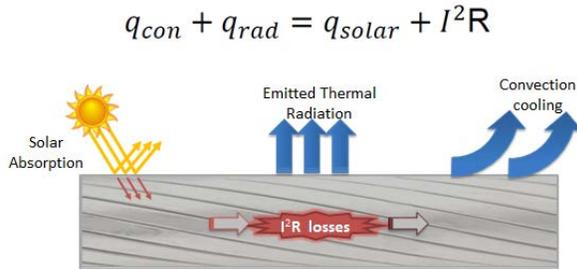
On the left side of the equation above is heat energy flowing out of the conductor from both convective and radiative cooling. On the right hand side is the heat generated in the conductor by electrical current and resistance plus the solar heat gain.
