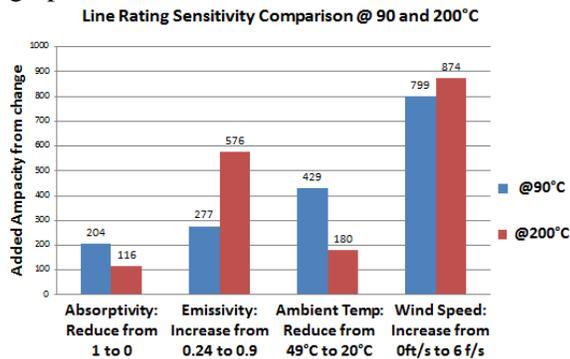
Note how at 90°C the difference between the impact of emissivity and absorptivity is 73 amps, while at 200°C, the difference is five times greater at 460 amps. The changing magnitude of these impacts has considerable implications for line rating risk and will be explored in more detail.
