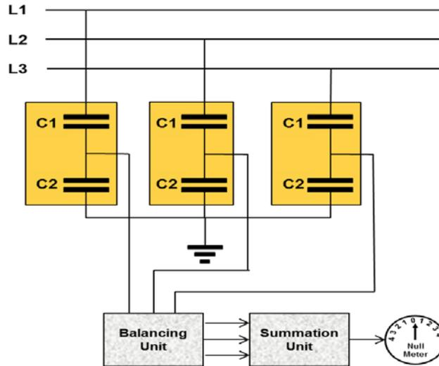
Figure 8: Principle of balanced current method
