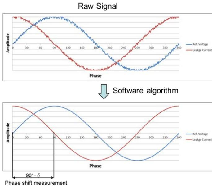
Figure 10: Example for effective noise elimination
