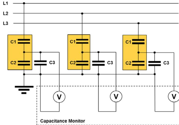
Figure 7: Principle of capacitance method
