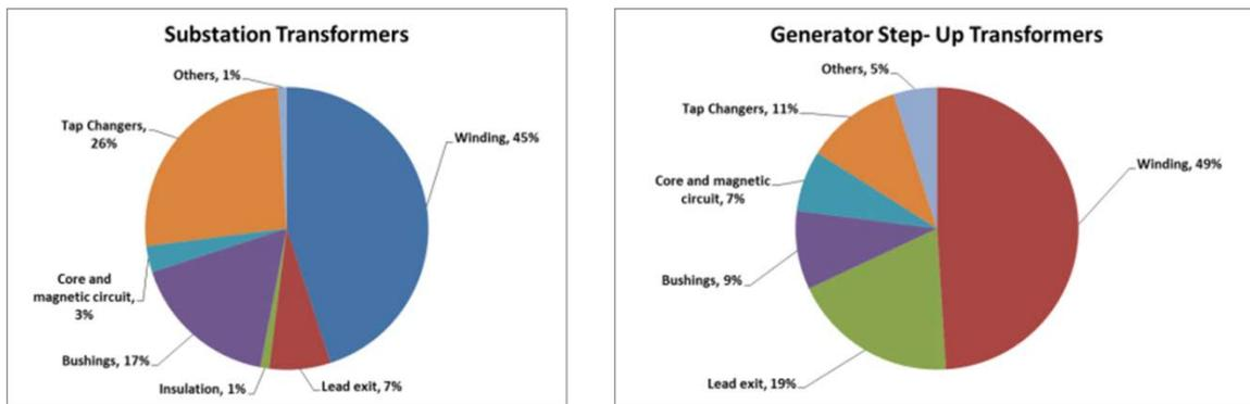
Figure 2: Failed component statistic
