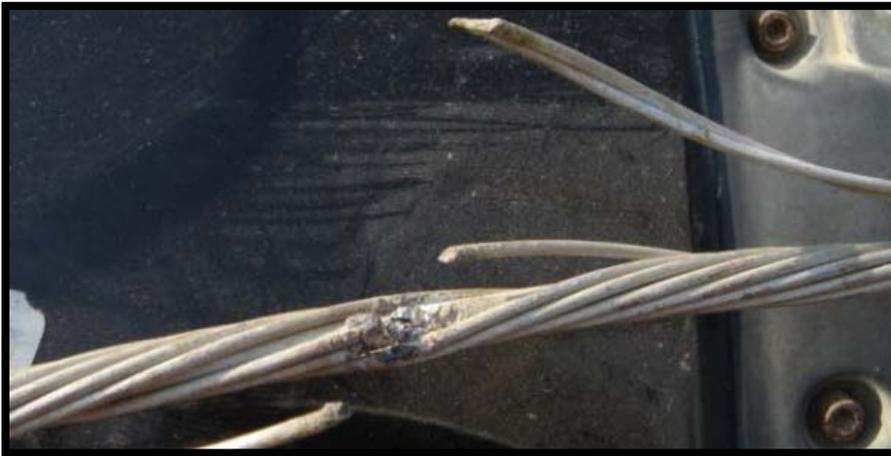
Figure 9. Lightning strike damage on transmission line shield wire.
