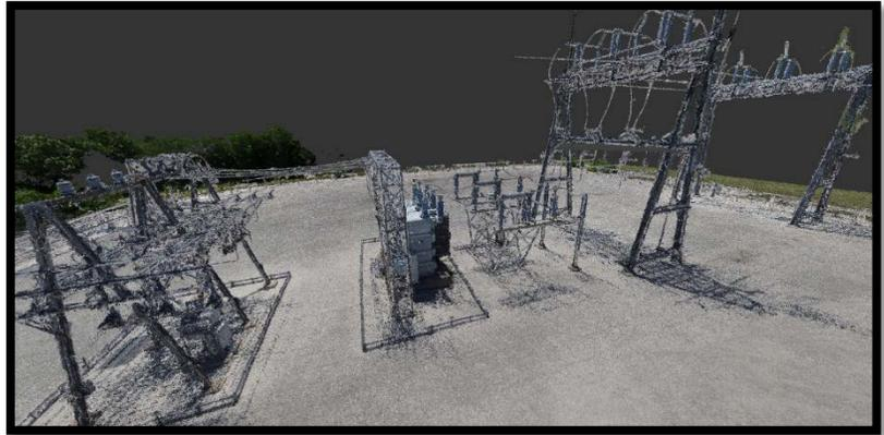
Figure 5. 3D point cloud using LIDAR
