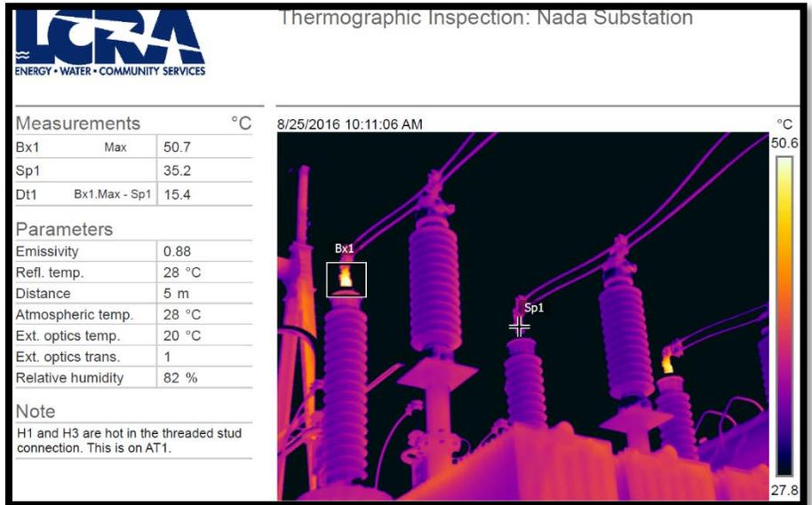
Figure 7. Infrared image of an abnormal connection at an autotransformer
