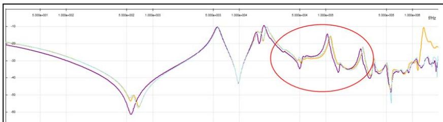
**Figure 2 – SFRA Results LV Open Circuit Tests**
