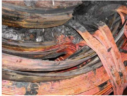
**Figure 3** – Observed Winding Movement LV Winding Phase B
