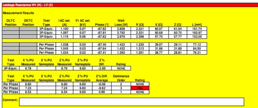
**Figure 1 - Leakage Reactance Results**
