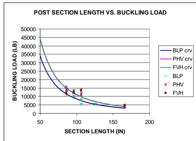
**Figure 6 - Plot of buckling loads by assembly type**
